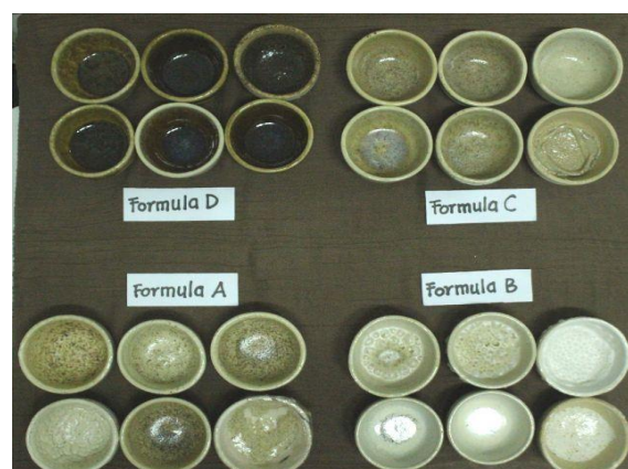
Figure 4. Bowl-shaped ash glaze test sample with 4 formulas. (Source: Caecilia tridjata suprabanindya, 2024)
