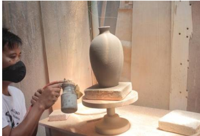
Figure 3. The process of coating the glaze on ceramic works uses the spray technique. (Source: Caecilia tridjata suprabanindya, 2024)
