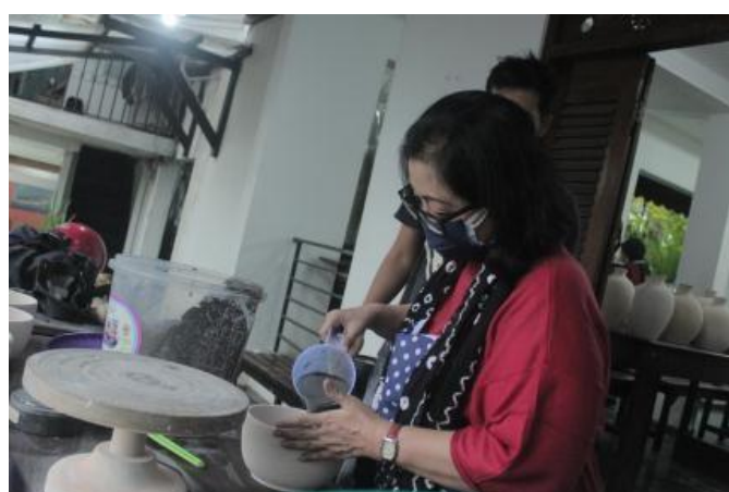
Figure 2. The process of coating the glaze on ceramic works uses the dyeing technique. (Source: Caecilia tridjata suprabanindya, 2024)
