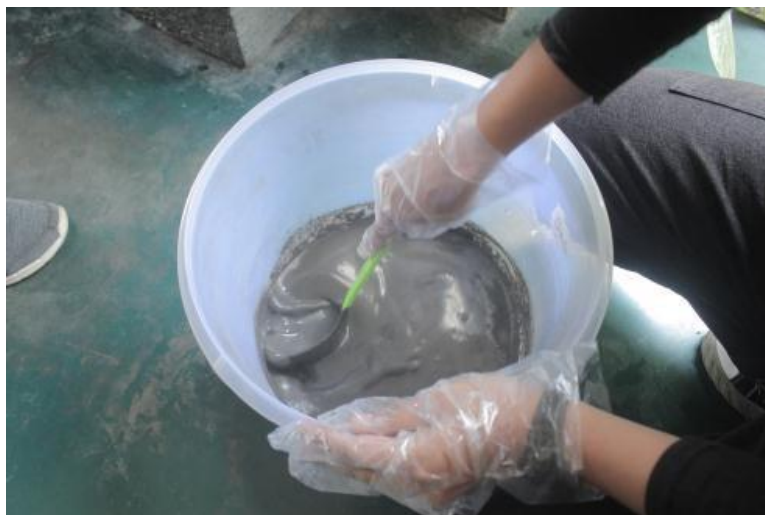
Figure 1. Manual mixing of jackfruit leaf ash glaze without ball mill. (Source: Caecilia Tridjata Suprabanindya, 2024)
