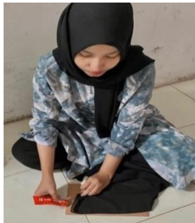
Figure 8. Process of Gluing the Lining to the Leather (Photo: Nuril Aulia, 2024)
