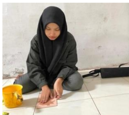
Figure 4. Process of Moistening the Vegetable Tanned Leather (Photo: Nuril Aulia, 2024)
