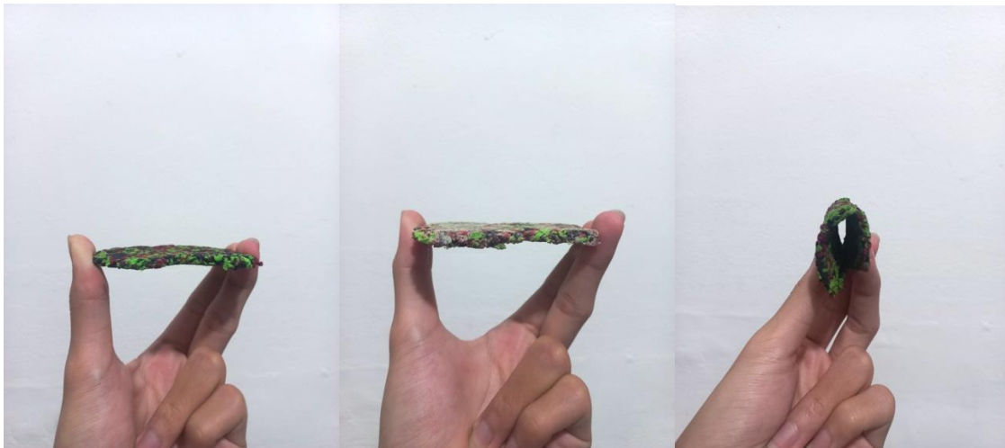
Gambar 4. Percobaan Bending (Lem PVAC – Lem Epoxy – Lem Chloroprene)
